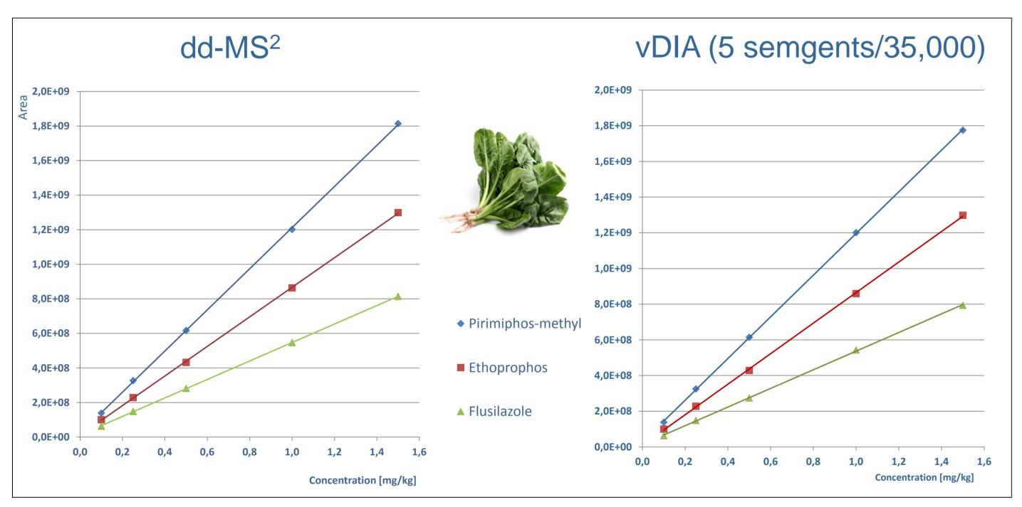
Independently of the workflow selected the detector response is characterised by very good linear range and no saturation is observed.
