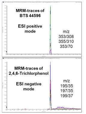
The chromatograms to the left demonstrate the insource fragmentation of BTS 44596 to TCP. Injection of a fresh BTS 44596 solution resulted in a peak at the MRM-traces of TCP but at the retention time where BTS 44596 is expected rather than where TCP is expected. This indicates an in-source fragmentation of BTS 44596 to TCP. To ensure correct detemination these two compounds they have to be separated chromatographically.
