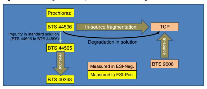
Although BTS 44596 is measured in the ESI-pos. mode, it is important to check its in-source fragmentation in the ESI-neg, mode to ensure that it will not co-elute with TCP or BTS 9608.
