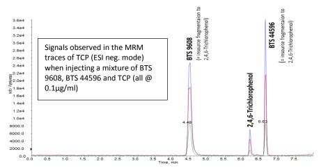
Interestingly the TCP-signals resulting from in-scource fragmentation of BTS 9608 and BTS 44596 were stronger than those obtained when injecting TCP itself at the same concentration
