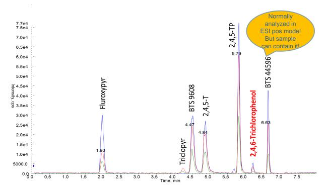
Also here the signal of 2,4,6-TCP is smaller than the signals produced by other similarly concentrated compounds via in-source fragmentation (all @ 0.1 µg/mL).
