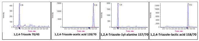
Figure 30: Typical chromatograms of TDMs in avocado extracts spiked at 0.01 mg/kg.
