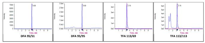
Figure 31: Typical chromatograms of DFA and TFA in tomato extracts spiked at 0.05 mg/kg
