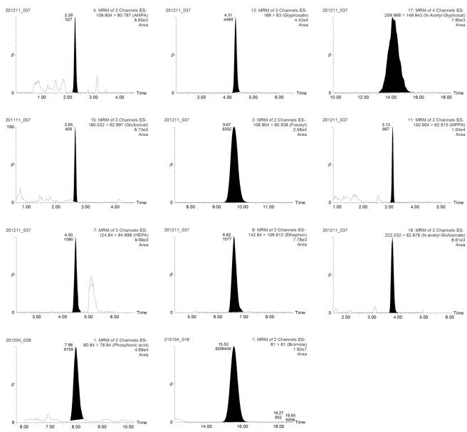
**Figure 13:** Chromatograms of Glyphosate, AMPA, N-Acetyl-Glyphosate at 0.06 mg/kg, Glufosinate at 0.036 mg/kg, HEPA, MPPA, N-Acetyl-Glufosinate at 0.024 mg/kg, Ethephon, Fosetyl at 0.012 mg/kg, all in strawberry extract and Phosphonic acid at 0.06 mg/kg, Bromide at 6 mg/kg both in lemon extract using <u>ii:</u> Waters Anionic Polar Pesticide Column, 130Å, 5  $\mu$ m, 2.1 mm x 100 mm.
