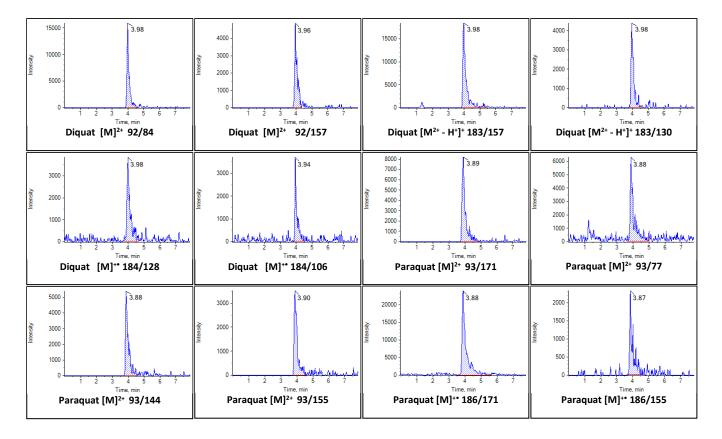
Figure 23: Typical chromatograms of Diquat and Paraquat in rice 0.005 μg/mL final extract (corresponding to 0,04 mg/kg)
