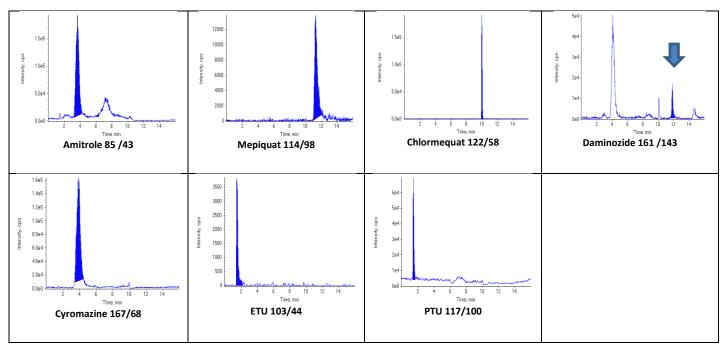
**Figure 21:** Typical chromatograms of Amitrole, Chlormequat, Mepiquat, Daminozide, ETU, PTU and Cyromazine in apple extract at 0.01 mg/kg
