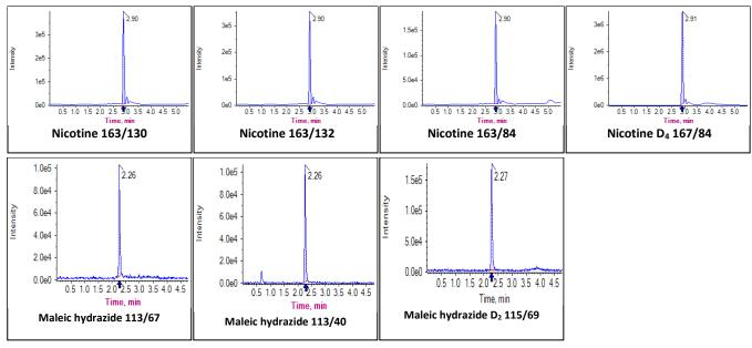
**Figure 25:** Exemplary chromatograms of nicotine in flour (spelt, whole-grain) Maleic hydrazide in solvent. Nicotine at 0.01 mg/kg (0.005  $\mu$ g/mL); nicotine D<sub>4</sub> at 0.1 mg/kg (0.05  $\mu$ g/mL); Maleic hydrazide and Maleic hydrazide D<sub>2</sub> at 0.2 mg/kg (0.1  $\mu$ g/mL).
