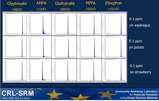
Figure 6: Typical chromatograms of Glyphosate, AMPA, Glufosinate, MPPA and Ethephon spiked on blank-QuPPe extracts
