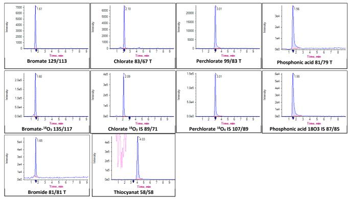
**Figure 10:** Chromatograms of Bromate (0.02 mg/kg) in currant extract, Bromide (1 mg/kg) in currant extract, Phosphonic acid (0.05 mg/kg) in currant extract, Perchlorate (0.01 mg/kg) in currant extract, Chlorate (0.01 mg/kg) in currant extract and Thiocyanate (1 mg/kg) in porree extract.
