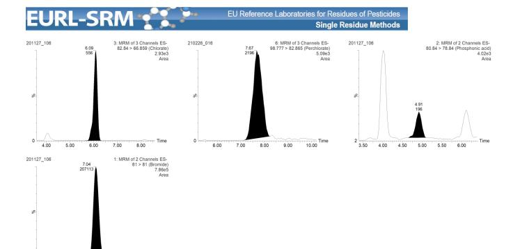
**Figure 15:** Chromatograms of Chlorate at 0.03mg/kg, Perchlorate at 0.01 mg/kg, Phosphonic acid at 0.05 mg/kg and Bromide at 5.0 mg/kg, all in lemon extract using <u>ii:</u> Waters Anionic Polar Pesticide Column, 130Å, 5  $\mu$ m, 2.1 mm x 100 mm; 50 °C.
