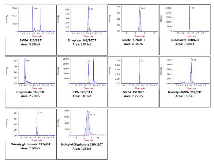
**Figure 12:** Chromatograms of Glyphosate, AMPA, N-Acetyl-AMPA, N-Acetyl-Glyphosate, Ethephon, HEPA, Glufosinate, MPPA, N-Acetyl-Glufosinate, Fosetyl at 0.04 mg/kg on cucumber extract using <u>i</u>: Waters Torus™DEA 2.1 mm x 100 mm .
