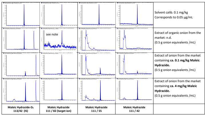
Figure 20: Typical chromatograms of Maleic Hydrazide in onion extracts and in solvent-based standards
