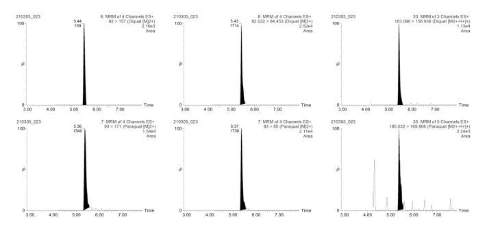
Figure 24: Typical chromatograms of Diquat and Paraquat in sesame extracts spiked at 0.05 mg/kg using Waters Xevo TQ-Sµ.
