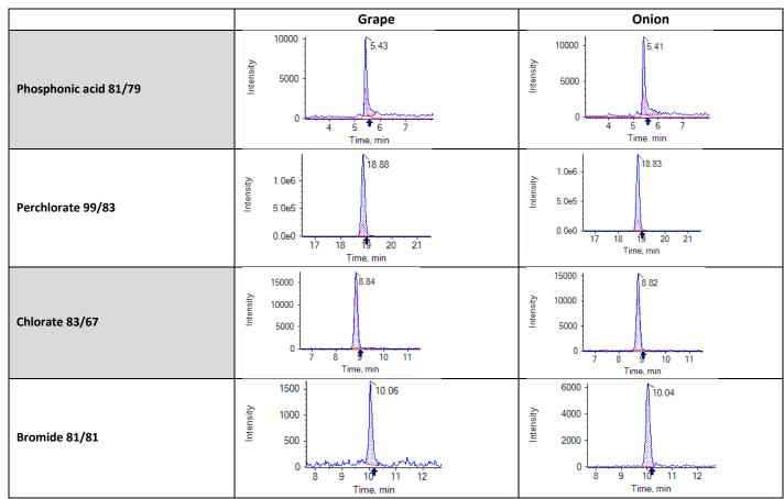
**Figure 16:** Exemplary chromatograms of Phosphonic acid, Perchlorate, Chlorate and Bromide at 0.01 mg/kg on Garpe and Onion using <u>i</u>: Waters Torus<sup>TM</sup>DEA 2.1 mm x 100 mm; 1.7  $\mu$ m; 50 °C.
