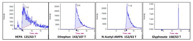
**Figure 3:** Chromatograms obtained using a new Hypercarb column, poor chromatographic behavior due to strong interactions of analytes with active sites. Same behavior is observed when the pre-column is new.
