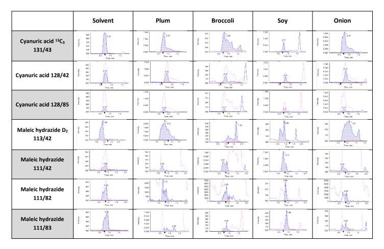
Figure 14: Exemplary peak shapes of Cyanuric acid and Maleic hydrazide in solvent-based standards and in standards of plum, broccoli, soy and onion extracts at 0.1 μg/mL (Please also read the note under "Hints on Method 1.6a and Method 1.6b" above)
