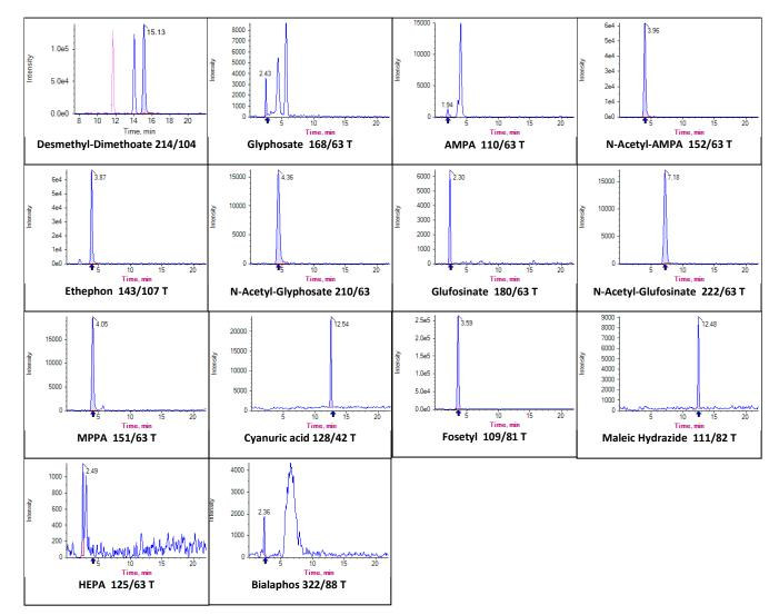
**Figure 9:** Chromatograms of Glyphosate, AMPA, N-Acetyl-AMPA, N-Acetyl-Glyphosate, Ethephon, HEPA, Glufosinate, MPPA, N-Acetyl-Glufosinate, Fosetyl, Maleic Hydrazide, Cyanuric acid and Bialaphos at 0.02 mg/kg on apple extract and Desmethyl-Dimethoate at 0.03 mg/kg on cherry extract.
