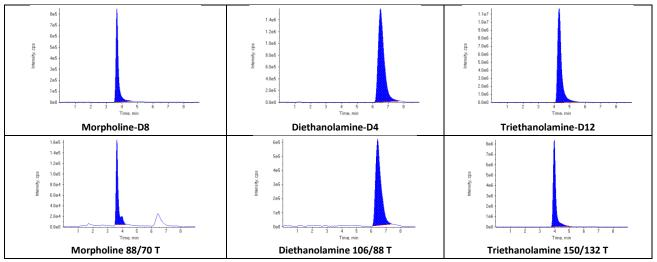
**Figure 29:** Typical chromatograms of Morpholine, Diethanolamine and Triethanolamine in apple extracts at 0.05 mg/kg (extract were diluted 10-fold before injection)
