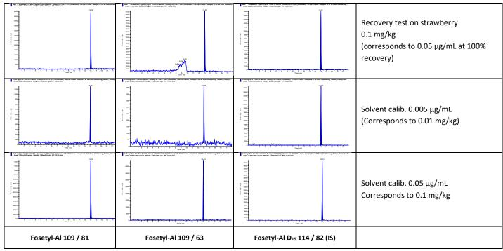
Figure 19: Typical chromatograms of Fosetyl-Al in strawberry extract and in solvent-based standards
