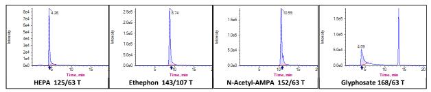
Figure 4: Chromatograms following priming with 25 injections QuPPe extracts of spinach. Injection volume 50  $\mu$ L per injection
