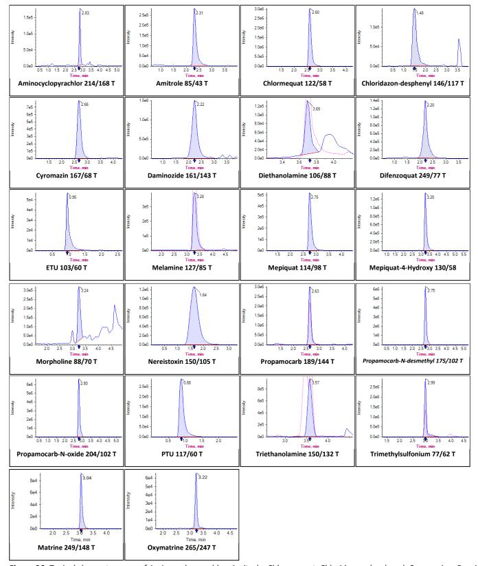
Figure 26: Typical chromatograms of Aminocyclopyrachlor, Amitrole, Chlormequat, Chloridazon-desphenyl, Cyromazine, Daminozide, Diethanolamine, Difenzoquat, ETU, Melamine, Mepiquat, Mepiquat-4-hydroxy, Morpholine, Nereistoxin, Propamocarb, Propamocarb-N-desmethyl, Propamocarb-N-oxide, PTU, Triethanolamine, Trimesium (Trimethylsulfonium) in tomato extracts spiked at 0.05 mg/kg; additionally Matrine and Oxymatrine at 0.01mg/kg in grape extract.
