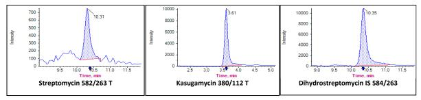
Figure 28: Typical chromatograms of Streptomycin and Kasugamycin in apple extracts spiked at 0.01 mg/kg.
