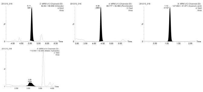
**Figure 17:** Chromatograms of Chlorate at 0.03mg/kg, Perchlorate at 0.01 mg/kg, Cyanuric acid and Maleic hydrazide at 0.05 mg/kg, all in lemon extract
