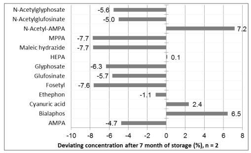
**Figure 36:** Deviations of the concentration of Glyphosate & Co. compounds in a working solution of 10  $\mu$ g/mL water containing 10 % acetonitrile and 1‰ HCl conc. (v/v), following 7 months of storage at 6 °C. Compared against a freshly prepared standard of same composition
