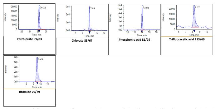
**Figure 34:** Typical chromatograms in milk extracts spiked at 0.01 mg/kg (Perchlorate and Chlorate); at 0.05 mg/kg (Phosphonic acid); 0.025 mg/kg (Trifluoracetic acid) and 5 mg/kg (Bromide).
