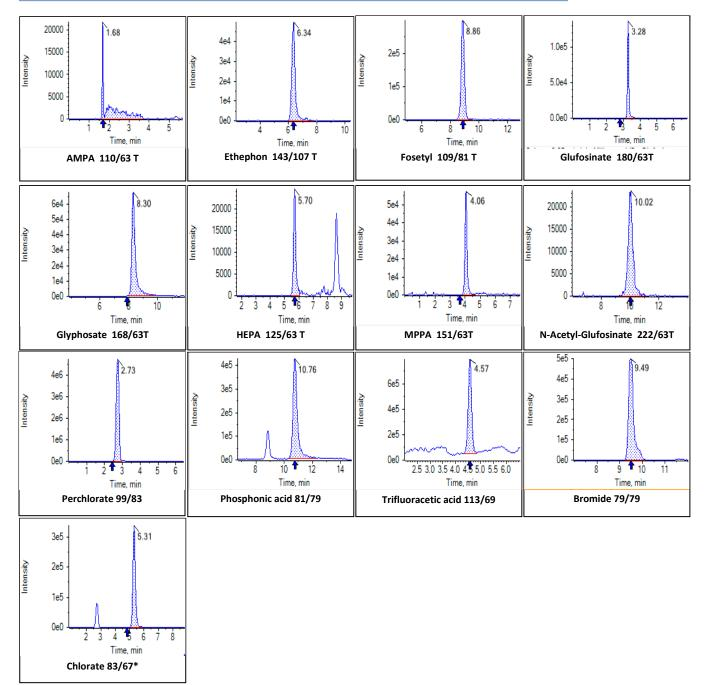
**Figure 18:** Typical chromatograms in strawberry extracts spiked at 0.1 mg/kg. \*for Chlorate matrix dependent retention time shifts were observed
