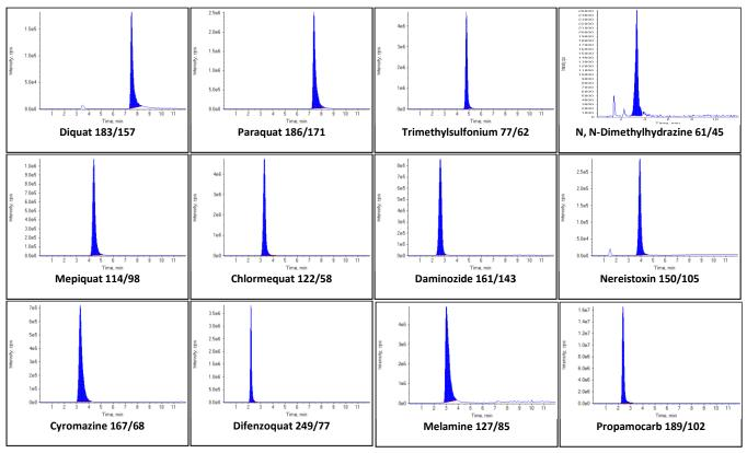
**Figure 22:** Typical chromatograms of Diquat, Paraquat, Chlormequat, Mepiquat, Daminozide, N,N-Dimethylhydrazine, Trimethylsulfonium, Cyromazine, Nereistoxin, Difenzoquat, Melamine and Propamocarb in apple extract at 0.1 mg/kg.
