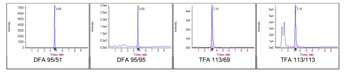
Figure 21: Typical chromatograms of DFA and TFA in tomato extracts spiked at 0.05 mg/kg.
