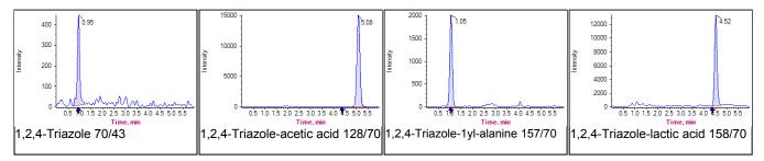
Figure 20: Typical chromatograms of TDMs in avocado extracts spiked at 0.01 mg/kg.
