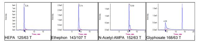
Figure 6: Chromatograms following priming with 25 injections (50 μL) of Spinach QuPPe extracts.
