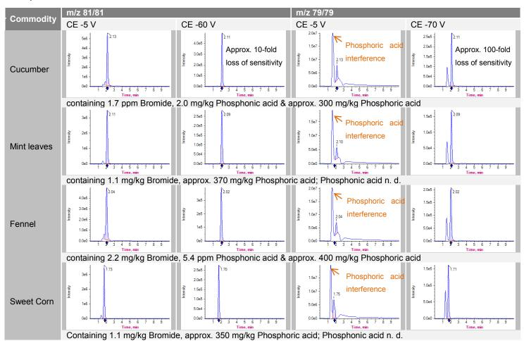
**Figure 12:** Chromatograms of Bromide using non-optimized collision energies (CE -5 V) showing the interference by Phosphoric acid and Phosphonic acid as well as optimized collision energies (CE -60 V and -70 V, the) showing reduced interferences.
