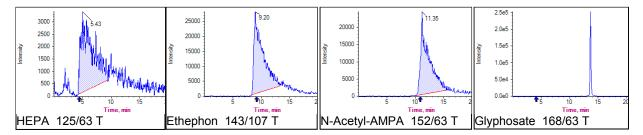
**Figure 5:** Chromatograms obtained using a new Hypercarb column, poor chromatographic behavior due to strong interactions of analytes with active sites. Same behavior is observed when the pre-column is new.
